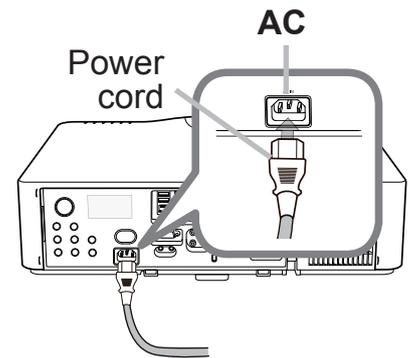
**⚠ WARNING** ▶ Do not connect the projector to a power supply while no lens unit is attached to it.
