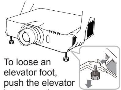
To loose an elevator foot, push the elevator button on the same side as it.
