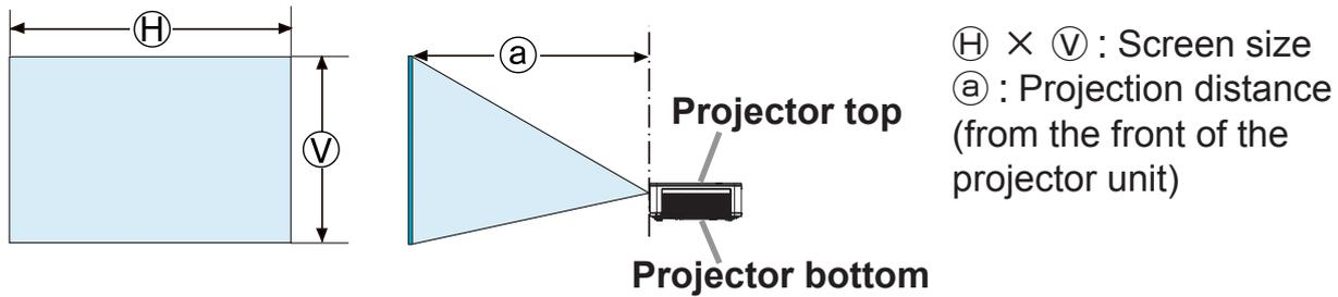
Secure a clearance of 50cm or greater between the exhaust vents and walls, and a clearance of 30cm or greater between the intake vents and walls. Assume that there is enough clearance in the front, back, and top of the projector in the figure below.
