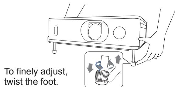
To finely adjust, twist the foot.
