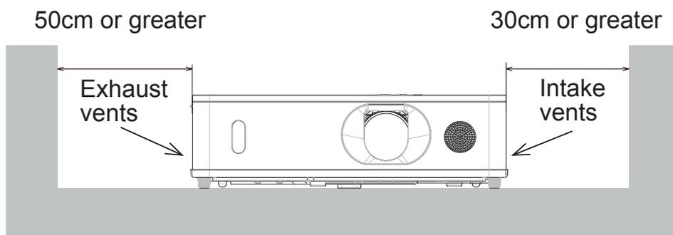
Secure a clearance of 30cm or greater between the intake vents and walls. Assume that there is enough clearance in the front, sides, and top of the projector in the figure below.
